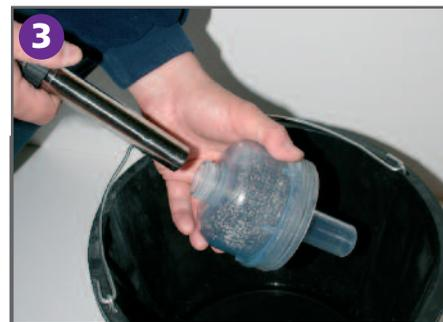
3 Once removed, place the clear base over a bucket. Unscrew and remove the magnet cap and rinse the sheath.
